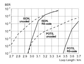
Fig. 2. Bit error ratio (BER) of uncoded and coded ADSL over POTS or ISDN (140 kHz), 2.048 Mb/s, 0.4-mm wire, 8 AslMx.
