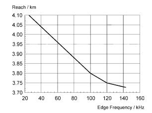
Fig. 1. Reach of the 2.048-Mb/s ADSL system dependent on the edge frequency  $f_e$  of the ADSL signal (0.4-mm wire, 1 AslMx).
